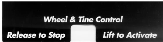
**WHEEL & TINE CONTROL BAIL:** Both decals describe operation of wheel & tine control. As the wheel & tine control bail is rotated rearward the wheels & tines will start rotating. The wheel & tine control bail is released and rotates forward the wheels & tines will stop but, the engine will continue operating.
