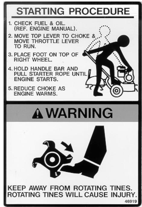
**STARTING PROCEDURE:** Describes procedure for starting tiller.
