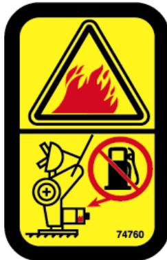
**WARNING:** To avoid fuel leakage and FIRE HAZARD, fuel must be drained from tank before standing tiller on end.
