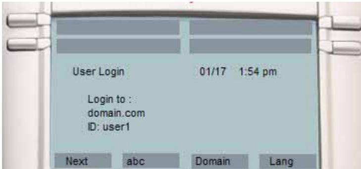
After you are logged in, the IP Deskphone displays the Idle screen. You can configure up to five profiles. If the limit is exceeded, then the least recently used profile is automatically deleted.
