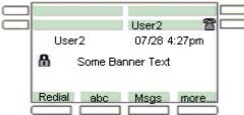
[Figure 8 on page 66](#) is an example of a secure connection when you are on an active call. The security icon is visible on the IP Deskphone screen.
