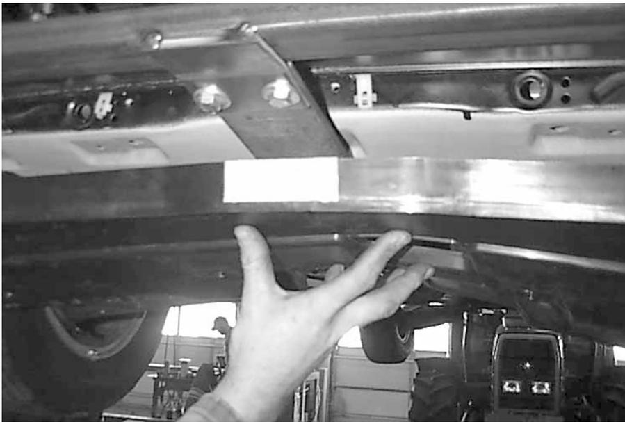
5. Trim splash shield according to photos and install. **Note: Lower photos show where ears of splash panel will have to be trimmed off.**
