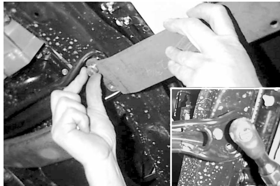
4. Install center support brace by taking two bolts out of vehicles center brace. **(NOTE: Be sure to leave in the third bolt, only remove two bolts.)** Attach center support to vehicle using two 10mm x 1.25 x 30mm bolts and 10mm lockwashers. Snug tighten these bolts and secure front of support using two 3/8" x 1-1/4" hex bolts, lockwashers, flatwashers and hex nuts. Push cross member up and tighten all bolts.
