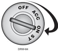
2. Enter 4-digit PIN code by turning the ignition On.
