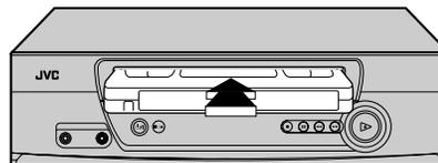
Make sure the window side is up, the rear label side is facing you and the arrow on the front of the cassette is pointing towards the recorder.
