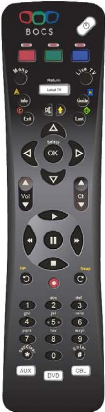
**Note** In step 1, if the LEDs on Xtender stop blinking immediately upon release of the pair button, the maximum number of remotes have already been bound to this Xtender (12 are allowed). To un-pair all remotes and start over, press and hold the **BOCS Logo** button for 10 seconds.
