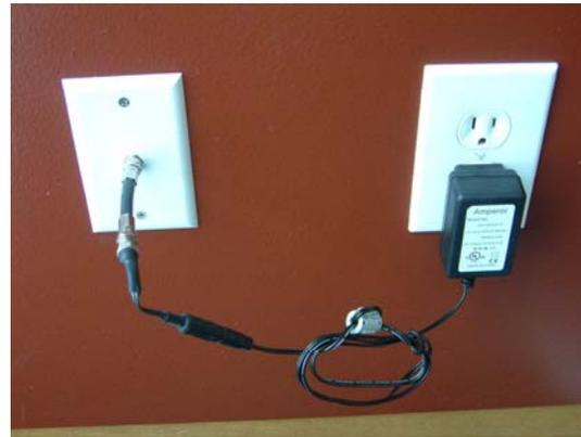
**Warning** – do not plug the coax adapter into a satellite TV outlet or you may damage your satellite TV system!!
