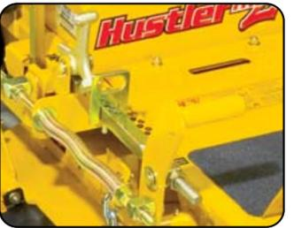
Spring-assisted, foot-operated deck lift for fast, simple adjustment of cutting height, negotiation of curbs, and movement on and off the trailer
