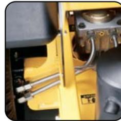
Stainless-steel high-pressure lines with Parker Seal-Lok™ O-Ring face seal fittings — no deterioration as with competitors' hoses
