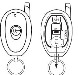
Carefully slide the two batteries out from under the clip in the direction indicated by the arrow.
