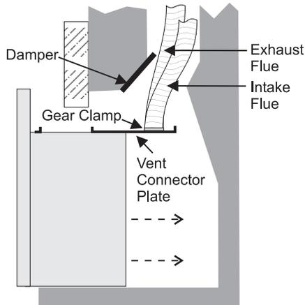
**Be careful not to damage thermal insulation when sliding on vent connector plate. This could cause blockage.**
