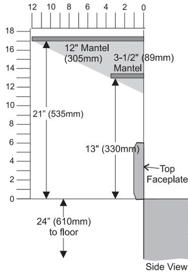
**Note:** A non-combustible mantel may be installed at a lower height if the framing is made of metal studs covered with a non-combustible board.
