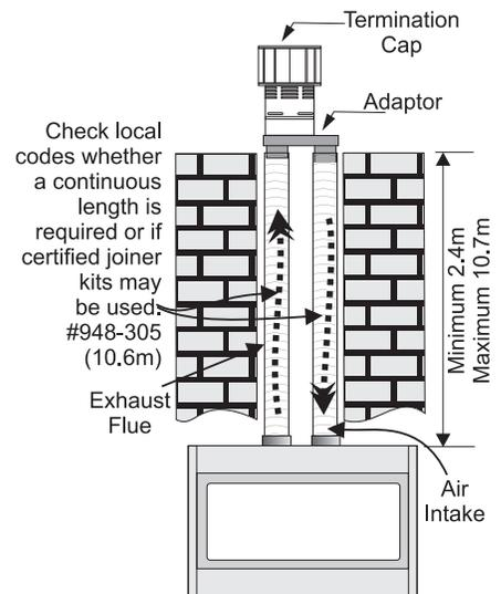
**Note:** When installing the flueing, identify the flues. Mark one exhaust and one intake as indicated on the top of the unit.
