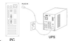
or other large electrical devices SHOULD NOT be connected to the UPS. Please make sure that the total loads of your equipments are less than the maximum total power load of your UPS.
