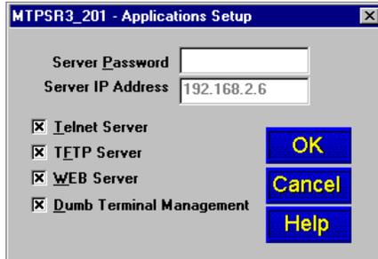
Enter a valid **Server Password** and **Server IP Address** (the IP address of the ProxyServer) and then verify that the desired applications are enabled. By default, the ProxyServer supports Telnet, TFTP, WEB, and Dumb Terminal management. If you wish to disable any of these applications, click the corresponding check box to disable support.
