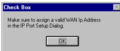
Click **OK**. This value was assigned in the initial software installation and was downloaded to the ProxyServer at the end of the installation. If you wish to verify or change the WAN IP address, click on **IP** in the **Firewall Setup** menu.
