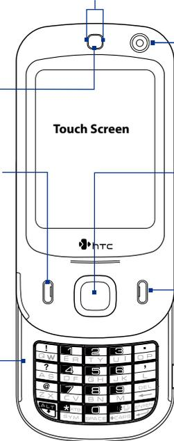
\* Right LED: Shows Green and Amber lights for HSDPA/UMTS/GSM/GPRS/EDGE standby, message, and network status as well as for notification and battery charging status. Shows a flashing red light when the battery level reaches 5% or lower.
