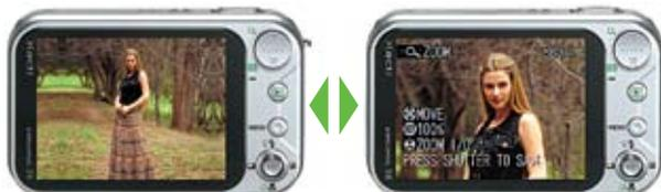
Snap a picture, and it takes just two quick button presses to zoom in and check the focus accuracy. The magnification ratio is automatically set according to the resolution of each photographed image for smooth checking of the image.
