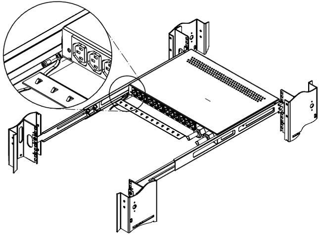
**Note:** The Ground Bonding wire must be a minimum of 10 AWG to maintain proper grounding.
