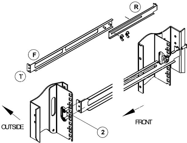
Use screws [1] (two on each side) to attach brackets to side of unit. Slide unit into rails and secure by using screws [2] (one on each side) to attach the unit.
