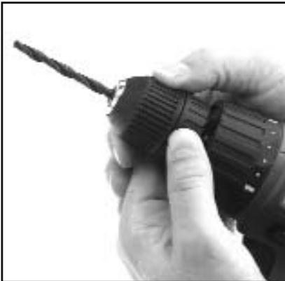
**Fig 1.** Inserting bits into the chuck.
