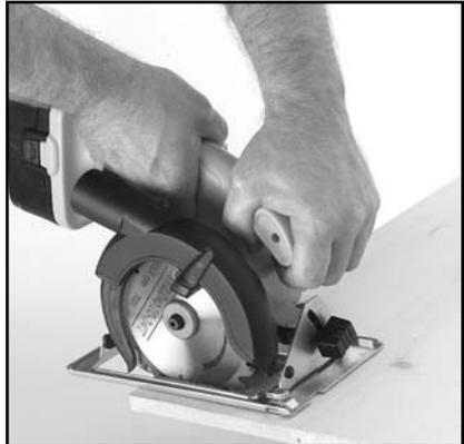
Fig 9. Proper Holding Grip.
