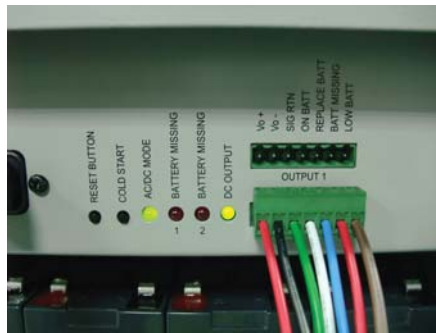
Figure 16: LED's and ONT Alarm Connections
