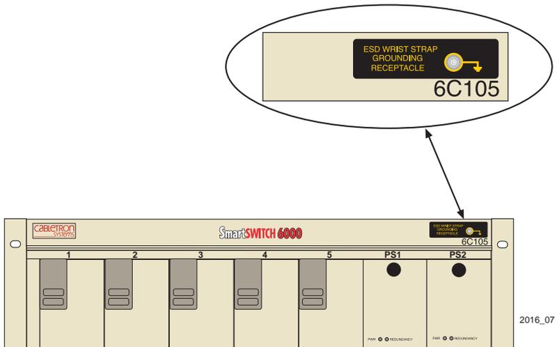
**Figure 3-3 ESD Grounding Receptacle**
