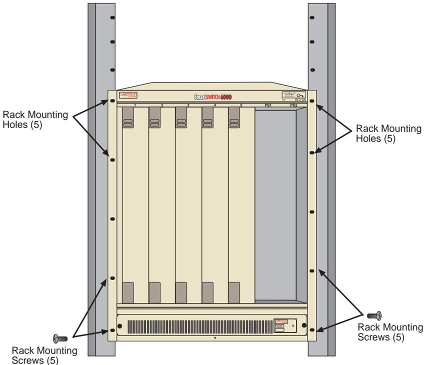
Figure 3-2 Rack Mounting the 6C105
