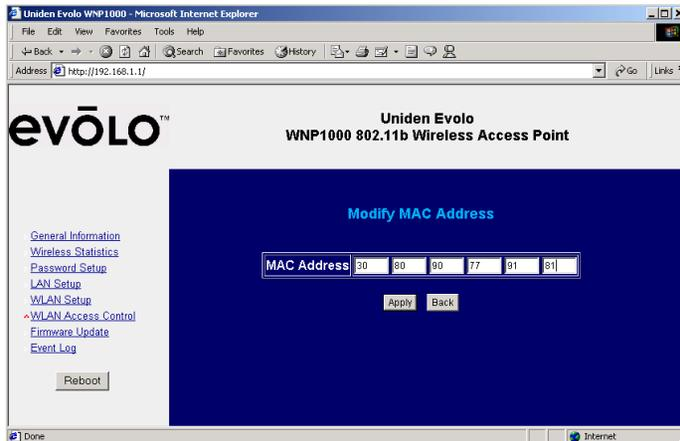
Uniden's client **MAC Address** can be found listed on the product label. For 802.11b clients, you can find the **MAC Address** listed on the package of the client network interface card. It consists of 6 pairs of characters, such as 00:30:AB:00:00:01.
