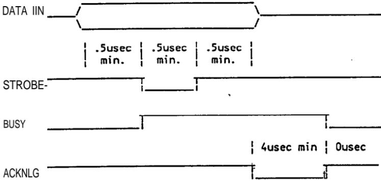
Data must be present a minimum of 0.5 u sec before and after a minimum 0.5 u sec STROBE Pulse. BUSY goes high before the end of the STROBE signal and remains high until the end of an ACKNLG pulse of minimum 4 u sec.
