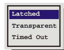
**Transparent:** The alarm is active only while receiving alarm input. The alarm condition is canceled when the alarm input ceases.
