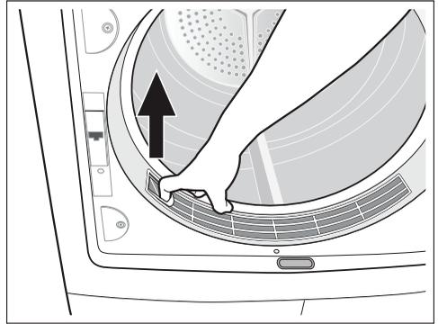
4. Push down the unlock button on the large mesh filter. The large mesh filter pops up.
