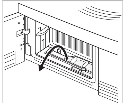
4. Use a damp hand to remove the fluff from the filter in the base. If necessary pull out and clean the filter with warm water using a wiper or brush. Clean the inside of the door, the fluff filter chamber and the rubber seals of fluff. Insert the fluff filter to the base.
