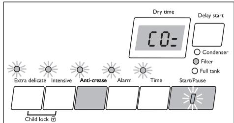
2. Press simultaneously the **Anti-crease** and **Start/Pause** buttons and hold down for approx. 5 seconds.
