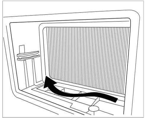
2. Pull the filter housing out of the base by the handle.
