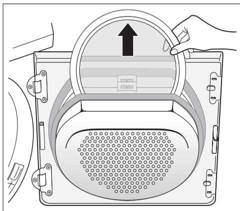
6. Remove the fluff from fine filter. It is best to use a damp hand for this purpose.
