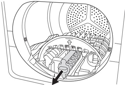
Loosen polystyrene parts 3 and 4.
