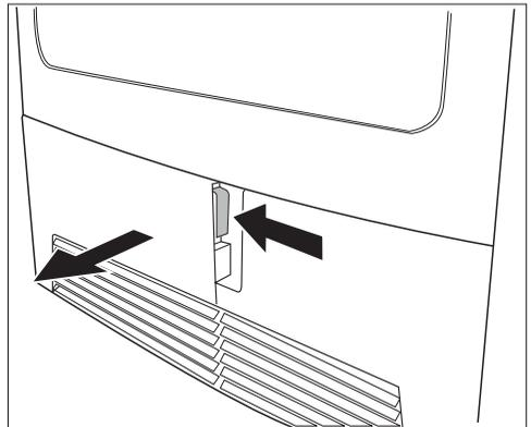
1. Open door in plinth: To do this, press the release button on the right and open the door in the plinth to the left.
