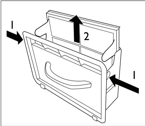
3. To clean the fluff filter: Remove filter from filter housing. To do this, press the pressure points on the sides and pull the filter frame up and out of the housing. Remove fluff from the fluff filter with a damp hand.
