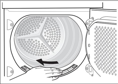
3. After a period of time, a gleam due to detergent residue on laundry forms on the filters. When this occurs, clean the filters with warm water using a brush. Remove the filter from the door pulling it out. (It can be positioned with the locating spur facing to the left or to the right). After cleaning do not forget to put it back.
