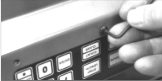
5. Lay module flat and remove the four screws from the back of the CPU and lift cover off.
