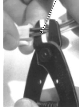
6. Remove the two hold-down clamps.
