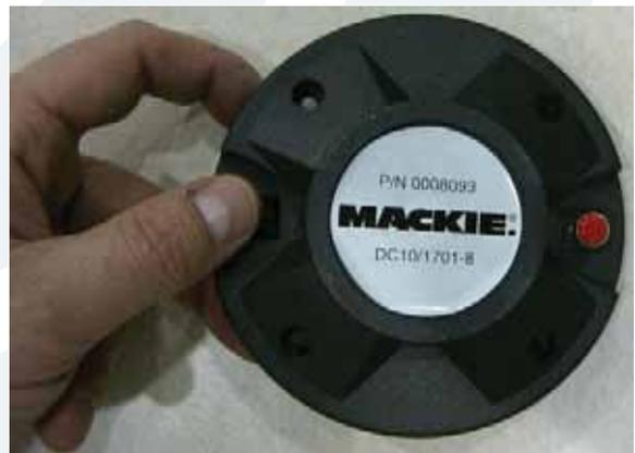
**6** This is what the plate adapter and diaphragm look like after they have been removed from the horn assembly. The diaphragm is separated from the plate adapter simply by pushing down on the terminals.
