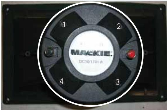
**3** The horn assembly is shown above with the high frequency driver circled. Four screws need to be removed from the driver using the 3mm allen wrench.
