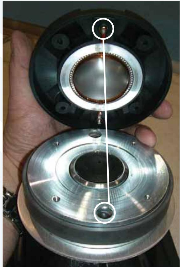
**5** The diaphragm and plate adapter are easily removed from the horn assembly. Notice the terminal locations in relation to the indents of the high frequency driver (circled above).
