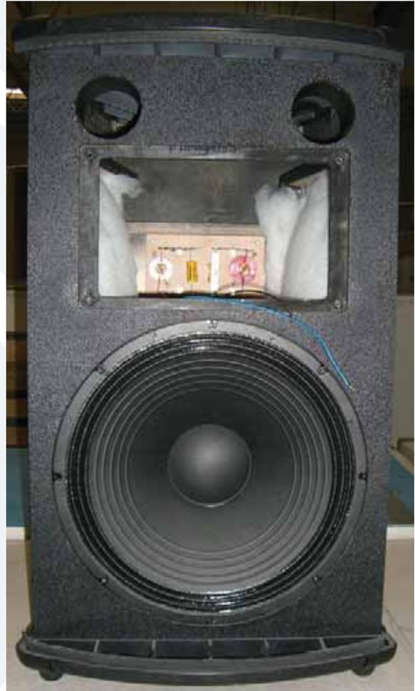
**7** This is what it looks like with the grill and horn assembly removed. See the next page for further instructions and additional pictures on how to remove and replace the high frequency driver.
