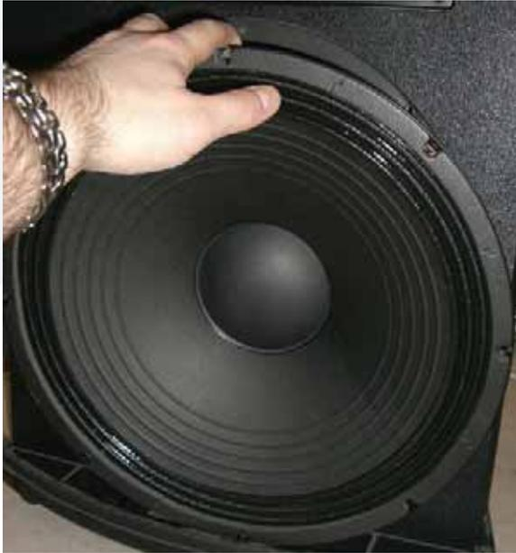
**5** Carefully begin to remove the woofer. This woofer has a tendency to want to pop out, so please be sure to hold the woofer in place with your free hand while removing the screws with the other hand.
