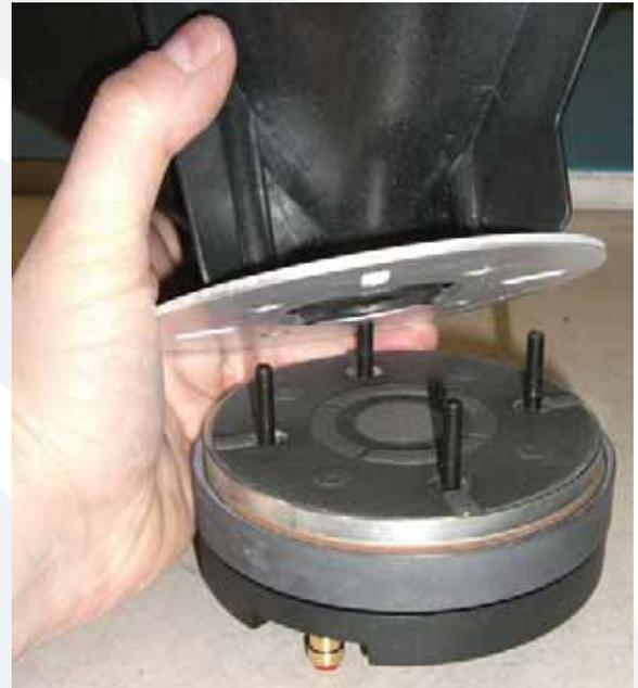
**8** Four nuts and eight washers may be removed from the driver using the 8mm open end wrench. Turn counter-clockwise to loosen and remove, clockwise to tighten. The other three are located around the horn assembly. Lift the horn up as the nuts are loosened. It cannot be removed otherwise. Notice that the flat washer is on the bottom, followed by the locking washer, and finally the nut.
