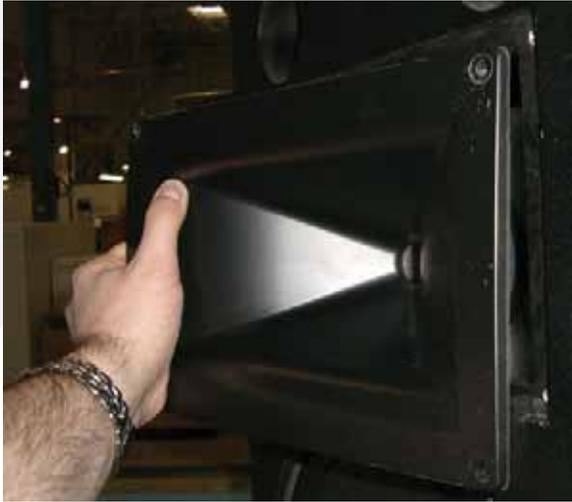
**5** Carefully begin to remove the entire horn assembly (with the high frequency driver still attached). A flat head screwdriver may aid in loosening the horn assembly by prying between it and the cabinet. Hold the horn assembly in place with one hand while prying around the edge with your free hand.
