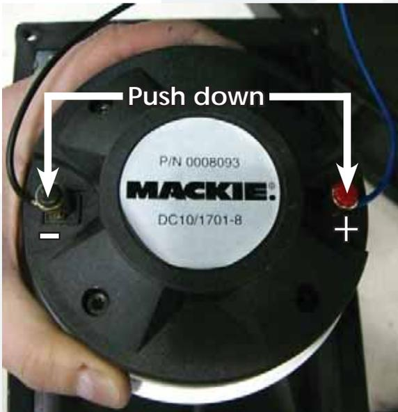
**6** The positive (solid blue) and negative (solid black) cables are still attached to the high frequency driver terminals. Remove the cables from their terminals simply by pushing down on the terminal and pulling out the cable.
