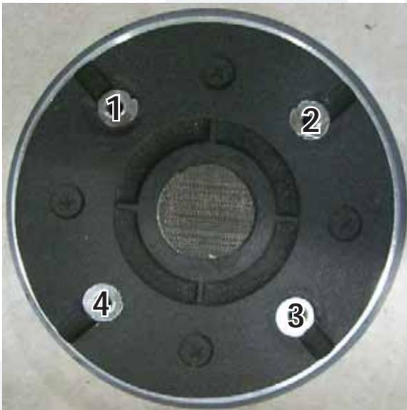
**12** Keep the four headless screws in a safe place. Place the new high frequency driver (part #0008093) where the old one was by following the same steps as above, but backwards 11 to 1. Power up the S215 and the new driver should now be pumping out those highs again. Fantastic, you just replaced a high frequency driver!
