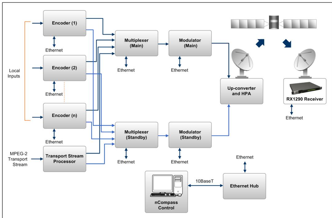
Figure 1.2 Typical Satellite Compression System
