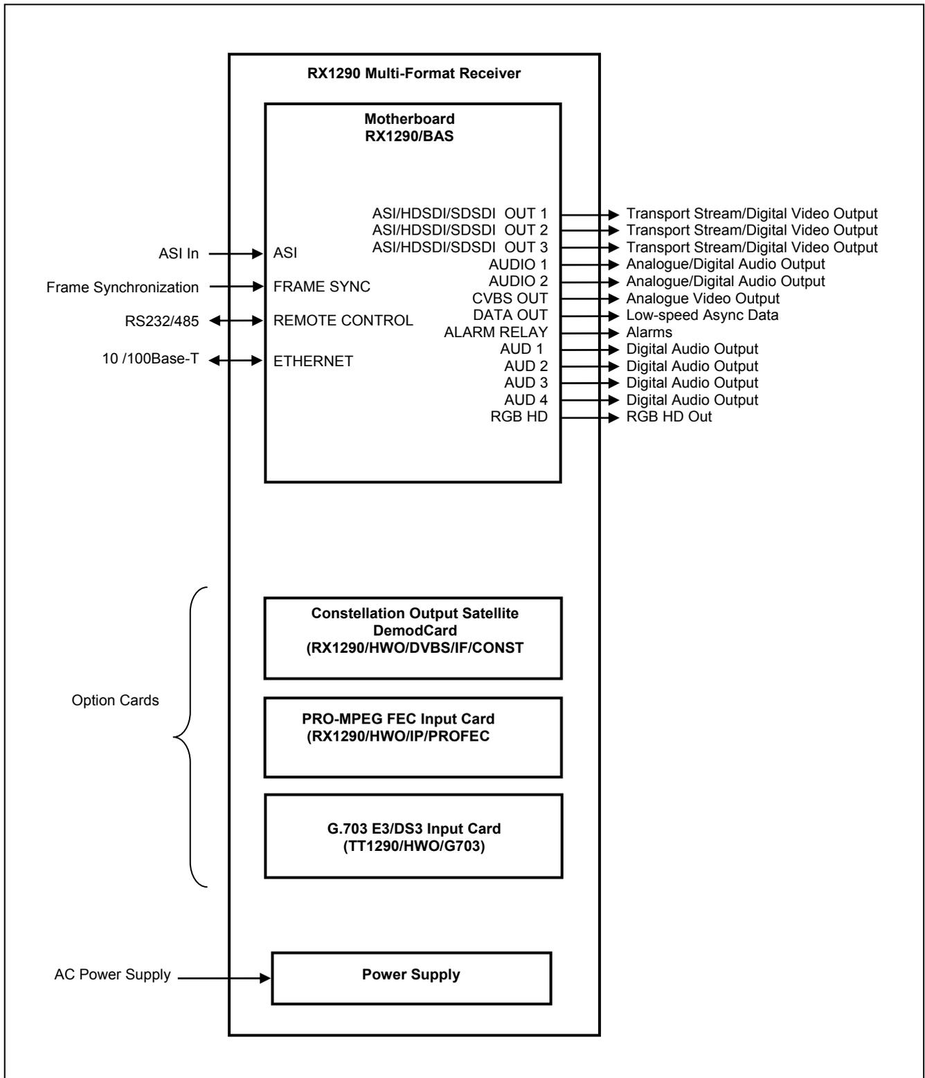
Figure 2.5 Signal Connections
