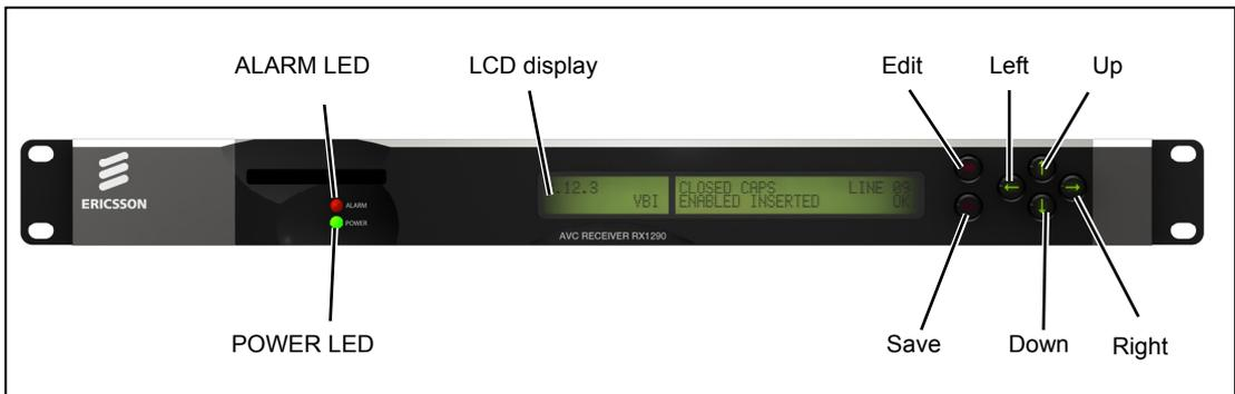
*Figure 1.7 Front Panel Controls*
