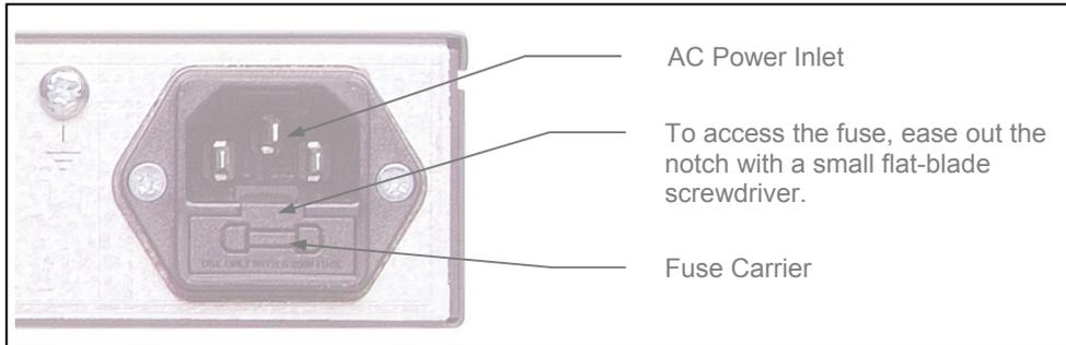
Figure 7.2 Fuse Carrier
