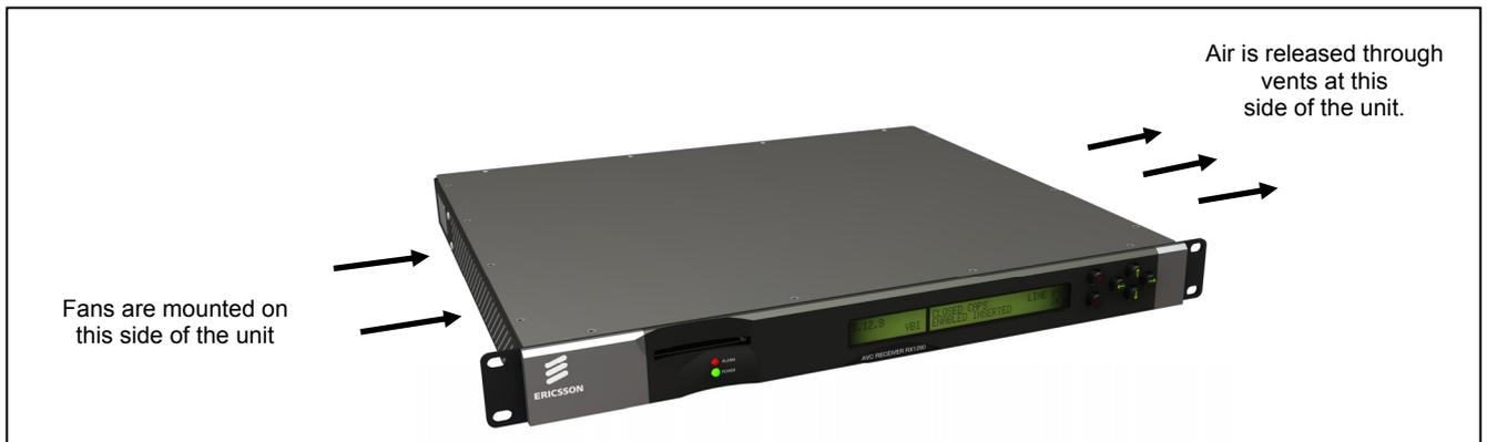
Figure 2.1 Air-flow Through the Equipment
