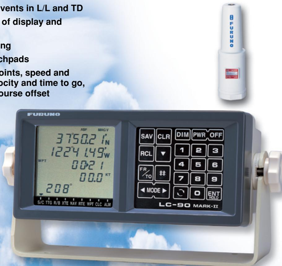
The FURUNO LC-90 MARK-II is a sophisticated hyperbolic navigation receiver accommodating all features necessary for safe and efficient navigation. It covers most Loran-C and Chayka stations in the world, complying with IMO and US RTCM Loran-C standards. Carriage of Loran-C and GPS navigators increases the availability of electronic position-fixing system (EPFS) for safety and efficiency at sea.
