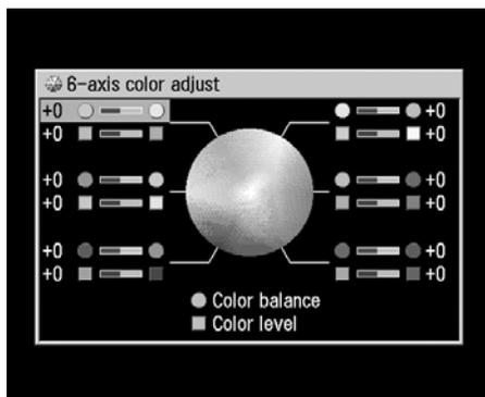
Select the "Color balance" or "Color level" bar using the [^] and [v] buttons, and then adjust colors using the [<] and [>] buttons.
