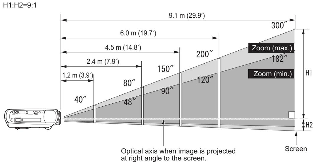
H1 and H2: H1 is the height of the screen from the intersection of optical axis and screen surface, and H2 is the height of the intersection when an image is projected at right angle to the screen.
