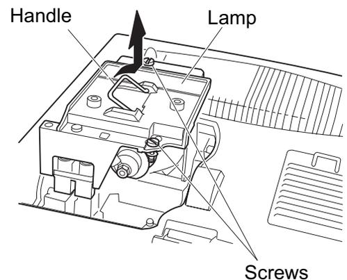
**4** Insert a new lamp as far as it will go and secure it with two screws.
