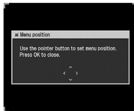
Using [^], [<], [>], and [v] buttons, move the menu position.
