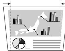
To reduce the length of the lower edge, press [v].
