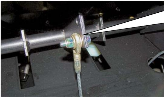
This center rocker arm lifts the front center of the deck. It also drops through the lower frame but is directed by two pulleys under the mower frame to the front of the deck.
