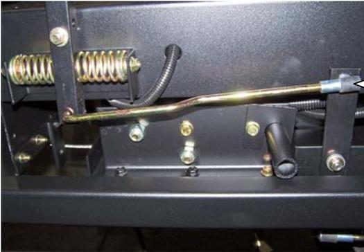
Once both hydro units are pulling equally, make your final control handle adjustment with this ball linkage. Whichever handle is going the farther forward, lengthen the linkage on that side until the handles are straight across when mower is traveling in a straight line. If a lot of adjustment is needed, shorten the linkage on the opposite side for half of the adjusting.
