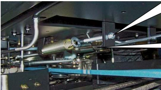
The deck lift system has two springs to assist in raising the deck. The ease of lifting the deck can be adjusted by tightening this nut equally on each spring.
