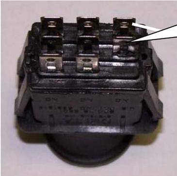
If all checked good in the two previous tests, the problem may now be a poor ground on the white wire in the clutch plug. Check by testing for continuity to ground or check for voltage between the two terminals
