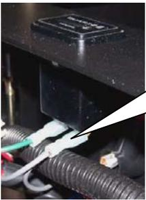
Hour meter has a **positive** and a **negative** post. Gray wire should go on the positive. Power is supplied from the ignition switch.
