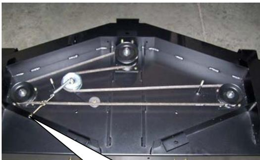
Tension on belt can be adjusted by tightening or loosening this nut.
