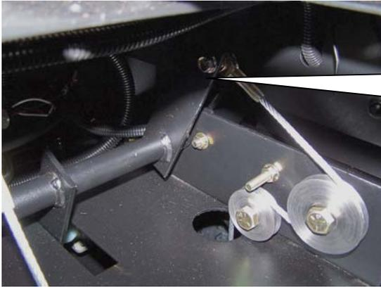
Three rocker arms are activated by the deck lift handle. This is the right side control. Note the routing of the cable. It drops straight below to the deck.
