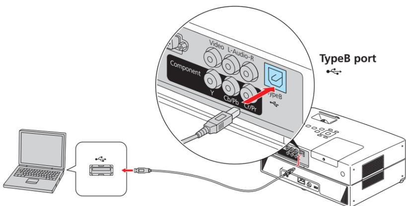
Follow the on-screen instructions to install the Epson USB Display software. (You need to install the software only the first time you connect.) After the software has been installed, you will see your computer's screen displayed by the projector.
