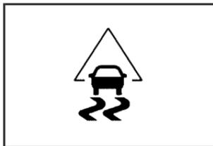
Your vehicle has a traction control system warning light.
