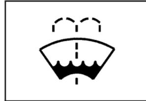
Open the cap with the washer symbol on it. Add washer fluid until the tank is full. See *Engine Compartment Overview on page 356* for reservoir location.
