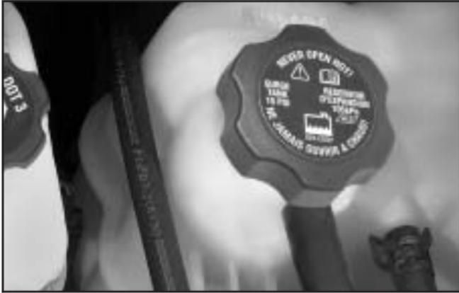
The coolant surge tank and pressure cap are located on the driver's side of the vehicle, toward the rear of the engine compartment. See *Engine Compartment Overview on page 356* for more information on location.
