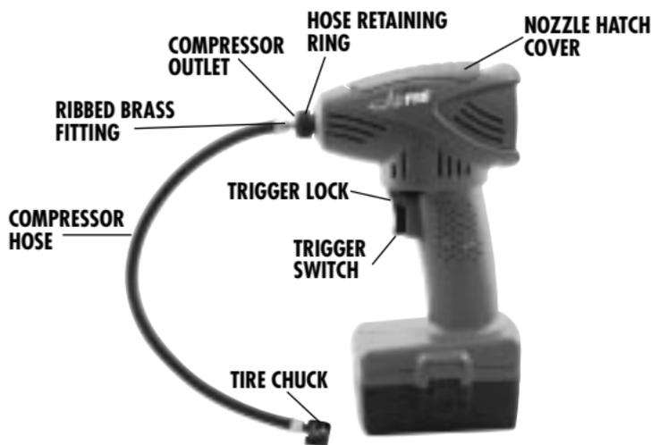
The Compressor On/Off Switch controls operation of the compressor. It conveniently is depressed and released to control inflation. An exact pressure is obtained by observing the gauge and releasing the trigger when the correct pressure is achieved. For longer inflation operations, the Trigger Lock can be moved laterally to lock the trigger in the ON position. Pushing the trigger lock to the opposite direction releases the trigger (OFF) and inflation stops.
