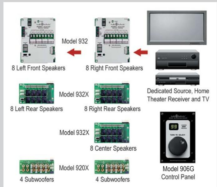
*This example system could switch up to eight speaker packages, each consisting of front, center and rear speakers, with subwoofer. The Model 906G Control Panel provides the ideal level of control for this simple switching application. Product select buttons could also be added to this system.*
