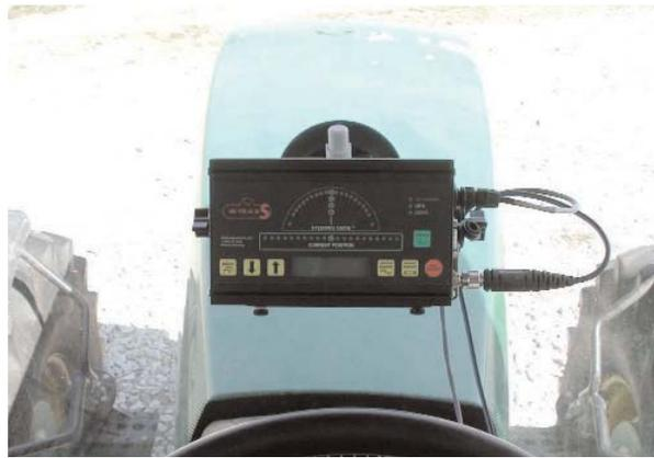
**4. Mount Display Unit:** THOROUGHLY clean the inside cab window surface directly in front of the steering wheel. Remove the red cover of the vacuum mount, press it to the window and pump the button located on the vacuum mount. Pump until the red line is no longer visible on the button. (Check it periodically. If the red line becomes visible, you may have to pump it a little to maintain suction). Adjust the display for proper viewing angle.
