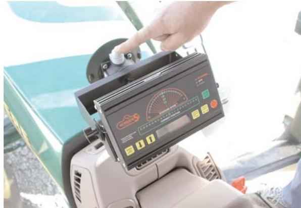
**NOTE:** Do not leave console unattended for extended periods of time. If possible, remove the unit from glass when not in use. Continued exposure to the elements (such as direct sunlight), can be harmful to the suction cup.
