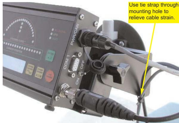
**NOTE:** Cigarette lighter sockets are *notorious* for intermittent power. For permanent installation, we recommend wiring directly to the battery, using a 5-amp inline fuse.
