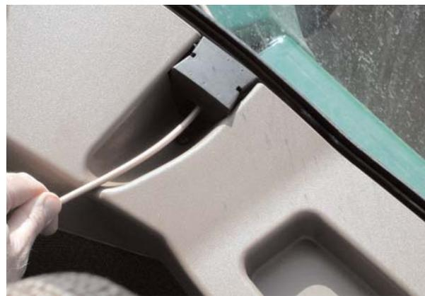
**6. Install Power Cable:** Connect the power cable to the display unit at the CAN port. Twist connector firmly until it snaps into place. For permanent installations, we recommend removal of the cigarette lighter plug and hard-wiring the leads to a reliable 12 volt power supply. Use a 5-amp inline fuse on the red lead to protect the console and wiring. Red goes to positive and black to negative. Coil excess cable in a protected location and secure the installation with tie straps.
