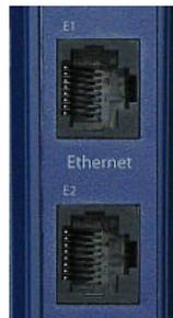
Figure 6. Ethernet Connectors. E2 is pass-through connection on model shown
