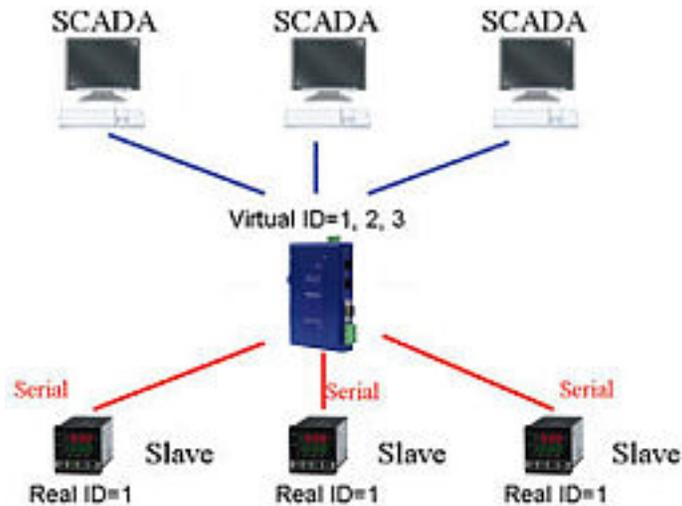
Figure 25. Scada to Slaves, IDs Fixed
