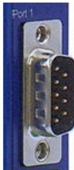
Figure 8. DB-9 Female Serial Port Connector
