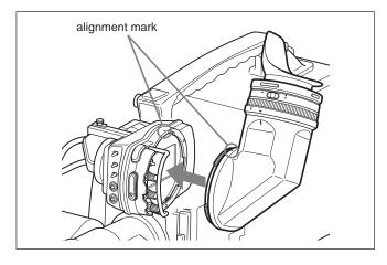
**2** Slide the viewfinder barrel into the body, while keeping the alignment marks aligned.
