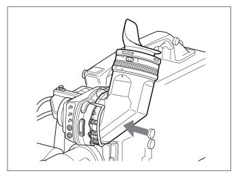
**3** Rotate the viewfinder barrel in the clockwise direction until the release knob clicks into place.
