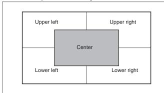
The center section is selected automatically the first time that you press the MAG button after powering the viewfinder on. Magnification does not affect the output signals of the camera.
