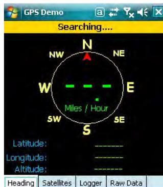
The yellow bar at the top of the window reads “Searching...” to show the GPS receiver is searching for visible satellites. When visible satellites are found, the Heading tab displays the exact position of the 9900.
