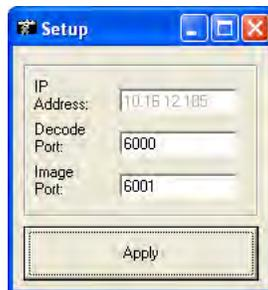
3. In the **IP Address** field, enter the IP address of the host workstation.
