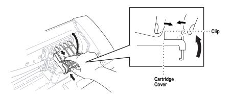
6 Remove the ink cartridge by lifting it up and out of the print head.
