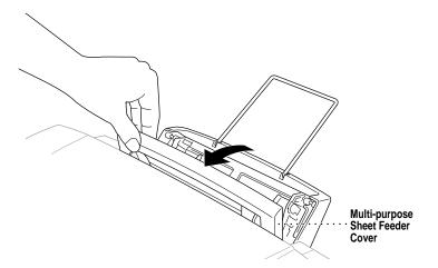
**B** Fan the paper well. Load the paper. Make sure the print side is toward you and the paper level is stacked below the paper guide line.
