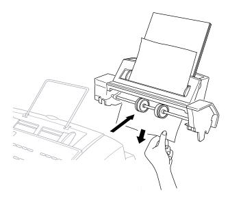
**3** Holding the cassette, pull the jammed paper out of the multi-purpose sheet feeder from underneath the cassette.
