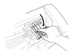
**10** After installing all ink cartridges, close the top cover until it clicks into place. Your MFC now prepares for a "head cleaning" and goes online so it can set the ink dot counter. The MFC will ask you if you changed each color ink cartridge.
