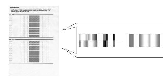
Using the Up/Down scroll control, select the best aligned print sample (1 to 9) for 360 and 720 dpi.
