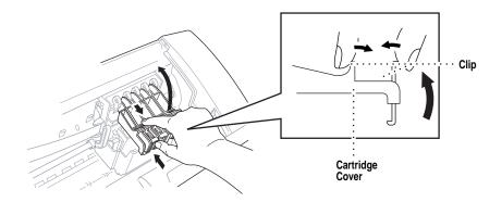
4 Remove the yellow shipping cover by lifting it up and out.
