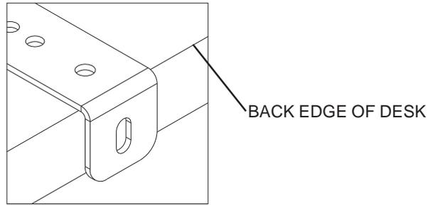
**7** Attach back lockdown brackets (**B**) to desktop using penta pin screws (**C**) at either location 1 or 2. Tighten securely with penta pin driver (**D**).
