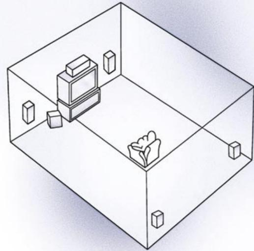
**Speaker Placement** After connection of the speakers place them so they appear in the approximate positions as shown in the diagram above.
