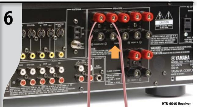
**Connect Surround Speakers** Positive (+) side of the wire with white stripe attaches to (+) terminal. Negative (-) side attaches to (-) terminal.
