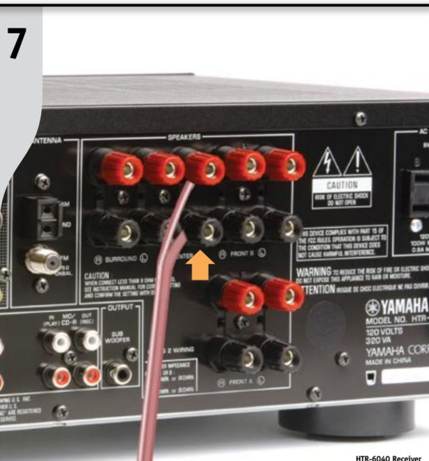
**Connect Center Speaker** Positive (+) side of the wire with white stripe attaches to (+) terminal. Negative (-) side attaches to (-) terminal.
