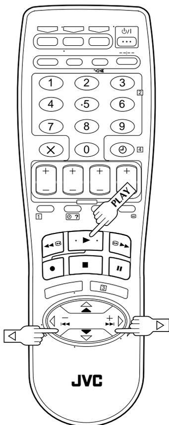
Your recorder is equipped with the TimeScan function. TimeScan allows noise free pictures to be displayed on your TV screen in the forward and reverse search modes. Audio will be played back at normal speed during the TimeScan modes (☞ pg. 19). TimeScan allows you to view a programme in search mode while listening to the audio.
