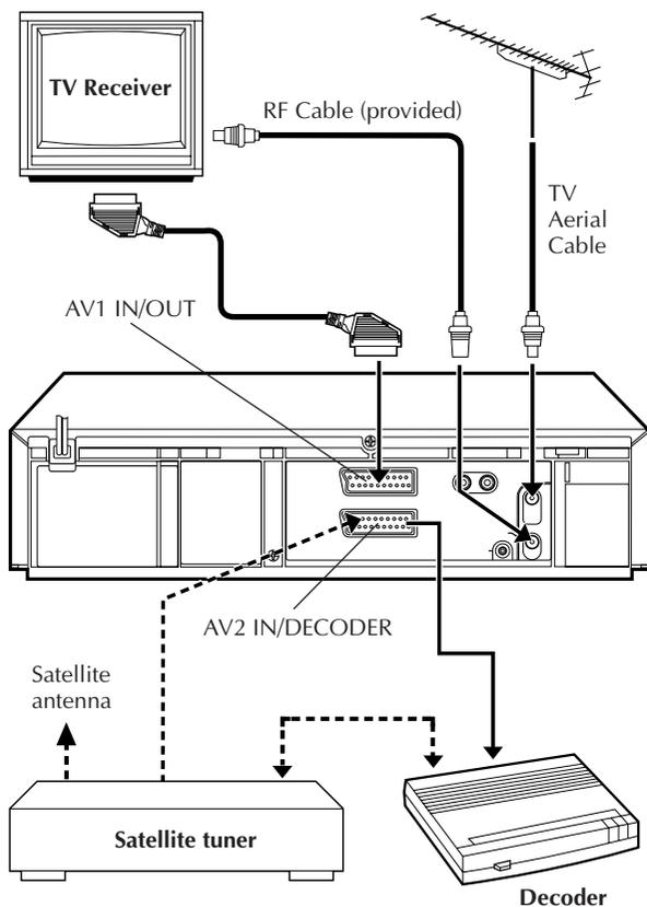
The AV2 IN/DECODER connector can be used as an input terminal for an external decoder (descrambler). Simply connect a decoder and you can enjoy the variety of programming that is available through scrambled channels.
