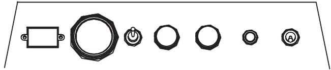
**11. RUN/STOP SWITCH** - RUN position energizes the engine prior to starting. STOP position stops the engine. The oil pressure interlock switch prevents battery drain if the switch is left in the RUN position and the engine is not operating.
