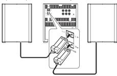
Connect the speaker cable plugs to the SPEAKER sockets.
