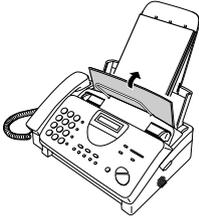
**Note:** When receiving faxes or copying documents, do not allow a large number of pages to accumulate in the output tray. This may obstruct the outlet and cause paper jams.
