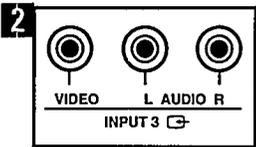
The VIDEO connection is a CVBS input. The AUDIO L and R inputs are for the sound from equipment connected to the VIDEO input.
