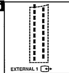
The Euroconnector is a multi-functional connection socket for both Audio and Video equipment (including RGB).
