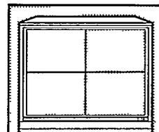
The cross which now appears on the picture should consist of a white horizontal and a white vertical line. If this is not the case and lines of different colours are visible, proceed as follows:
