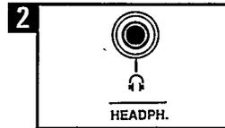
This connection is for headphones with an impedance of between 8 and 1000 ohms and is of the 6.3 mm Jack-type socket.
