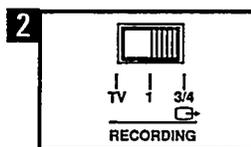
Via the RECORDING
