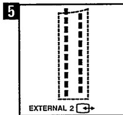
As an extra you can also connect a Eurocable, if the Video Recorder is supplied with a Euroconnector. The connection is made via Euroconnector EXTERNAL 2 (
