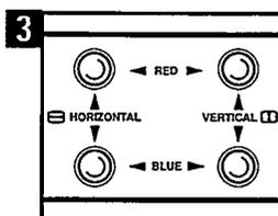
● Turn the buttons +/— RED HORIZONTAL ⊖ VERTICAL ⊞ so that the red lines coincide with the fixed cross already on the screen.
