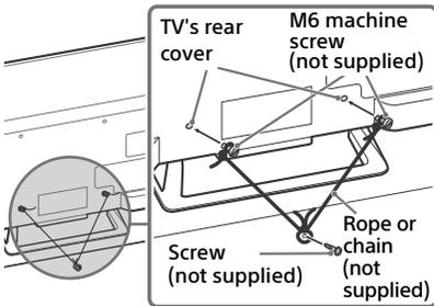
The length of the M6 machine screw differs depending on the rope or chain diameter. Please refer to below illustration.
