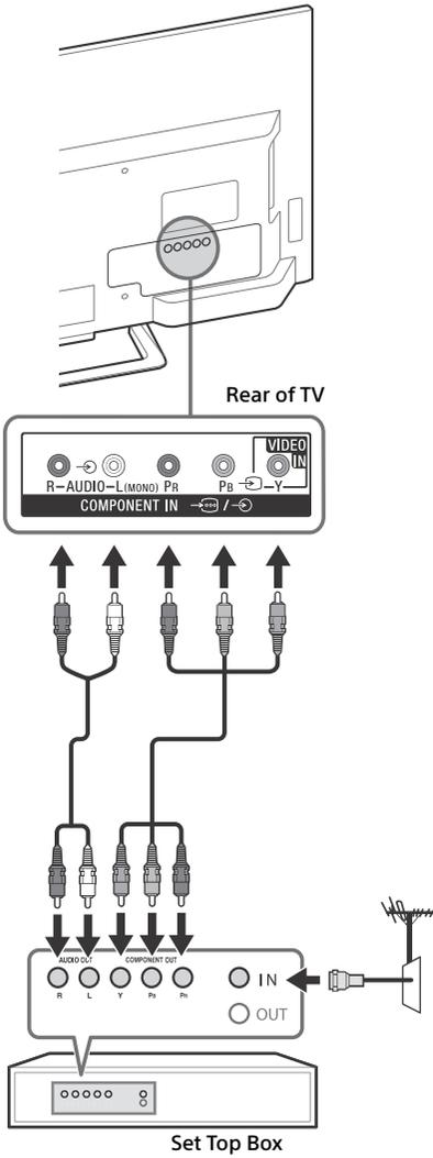
**Cable System or VHF/UHF Antenna System**
