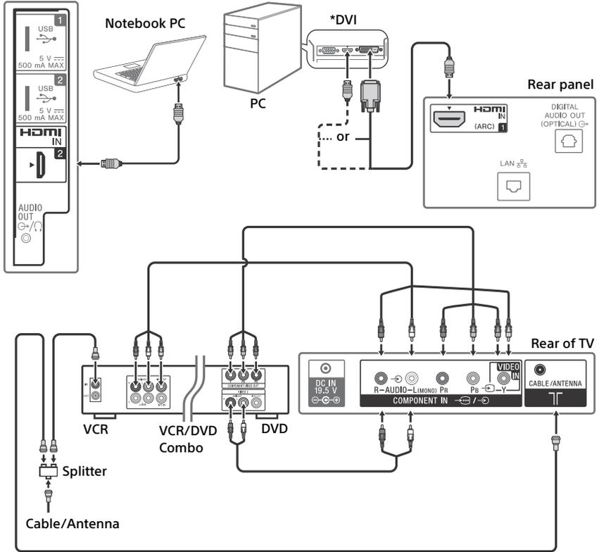
\* DVI does not support audio signals. Connect the audio output of the PC to the PC speakers or an A/V receiver to listen to sound from the PC.
