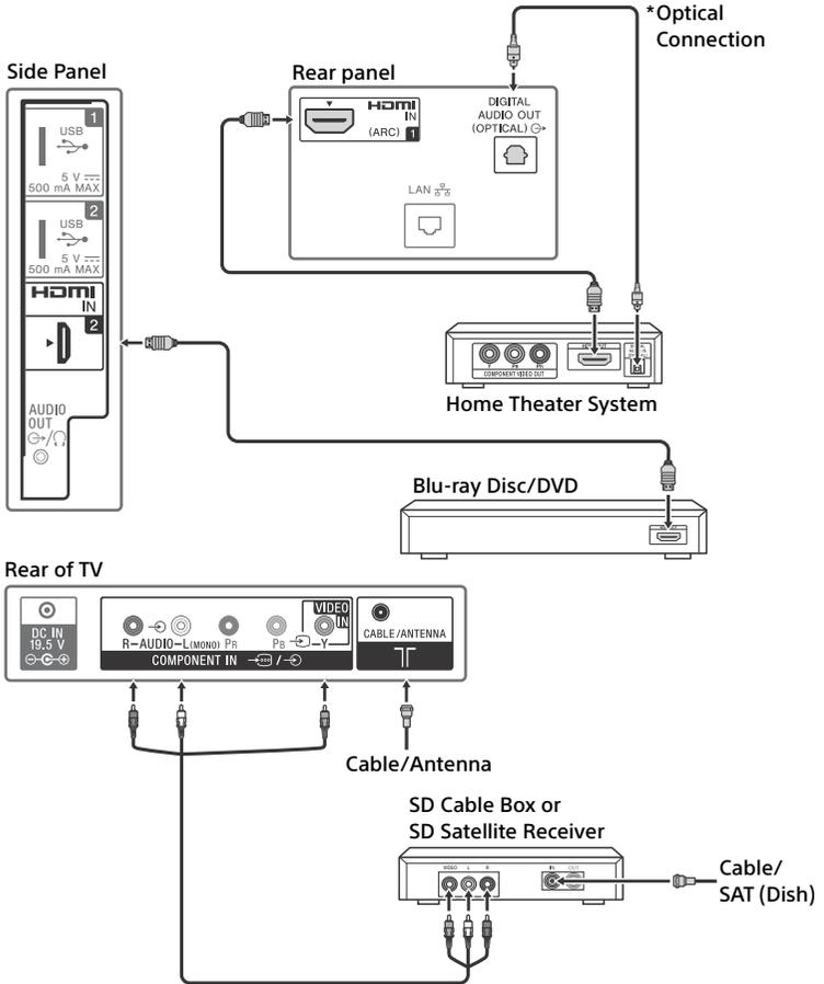
\* The optical connection is only needed for home theater system that do not support ARC (Audio Return Channel) when connecting with HDMI.
