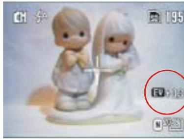
After you manually set the exposure value in "Manual" capture mode, the exposure value will be shown on the LCD screen.
