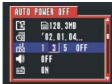
3. Then press the LEFT/RIGHT button (
