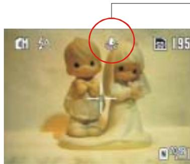
After you manually set the white balance mode in "Manual" capture mode, the following information will be shown on the LCD screen.
