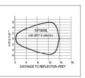
If the object that is to break the beam has a shiny surface, then the SP300L and its retroreflector should be mounted so that the beam is at an angle of 10 degrees or more to that surface in order to eliminate false signals which are caused by proxing.
