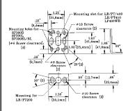
Accessory bracket model SMB300 is designed for 2-axis universal mounting of sensor models SP300EL, SP300RL, SP300L, and SP300D. These sensors are affixed to the SMB300 with two #6 (3,5mm) screws. The bracket, in turn, mounts with two #10 (5mm) screws.
