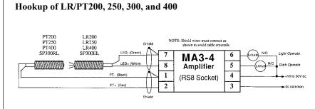
NOTE: Shield wires must be connected as shown to avoid cable crosstalk.
