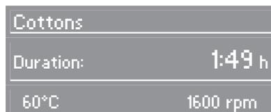
Pressing the left hand *Menu* button under **60°C** alters the temperature and pressing the right hand *Menu* button under **1600 rpm** alters the spin speed.
