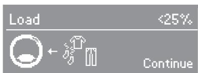
The display shows the amount of laundry loaded in the drum as a % (in 25% steps) of the maximum load permissible for the programme selected.
