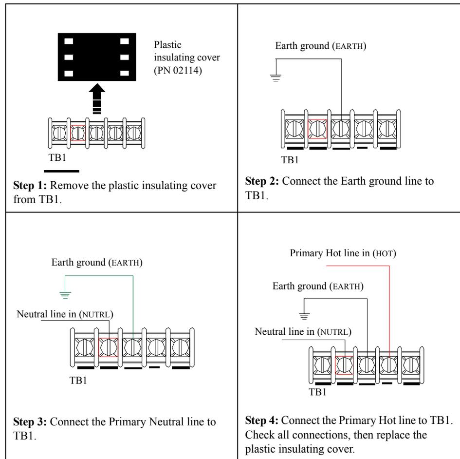
**Figure 4 Connecting AC Power to the Charger**
