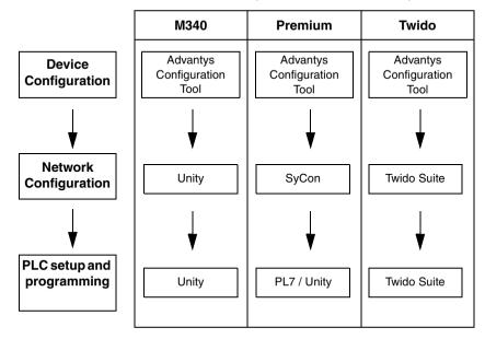
**Note:** With Twido Suite, Advantys Configuration Tool is run directly by Twido Suite to create or modify an island.
