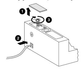
**Note:** Use a grounding strip or a conductor with a cross-section of 1 to 1.5 mm<sup>2</sup> (AWG18, AWG16) and a length of  $\leq$  3 m (9.84 ft) long. The maximum recommended length for the grounding strip is 3 m (9.84 ft).
