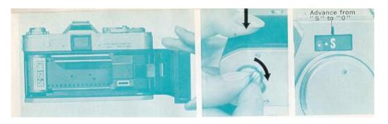
4. When the back cover is half closed, the QL cover presses down on the film. Check through the sprocket window whether the film has been engaged correctly onto the gear.
